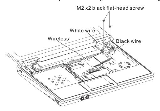
Figure 4-7 Removing the wireless LAN card
